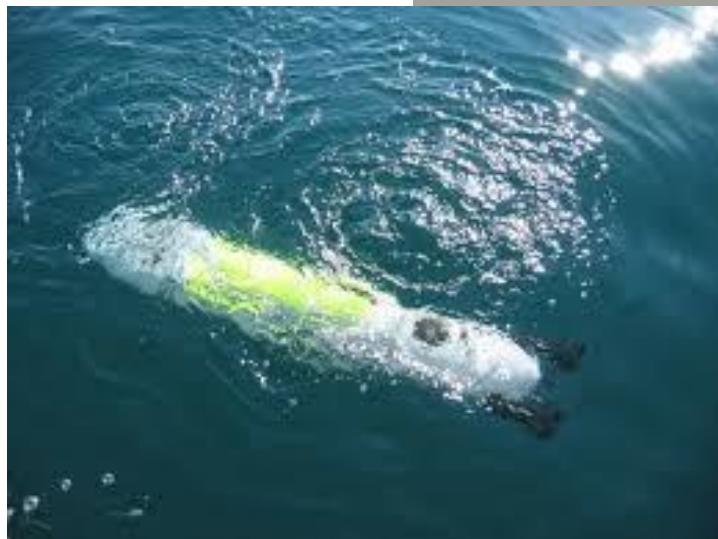
INESC TEC's Centre for Robotics and Autonomous Systems (CRAS) in Porto, Portugal, develops prototypes for the marine sector with hyperbaric test capacity until 250 bar for devices with volumes until 1000 mm length and 230 mm diameter. CRAS conducts research and development activities in autonomous robotic systems, mobile robotics, among others.
